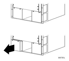
1. If necessary, remove the filler panel from a power supply bay.
